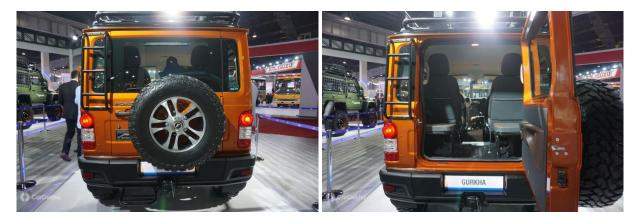
There is a step at the back for passengers to get in and out of the rear door comfortably. The toe-hook next to it means business, allowing for the Gurkha to tow another vehicle quite easily.
