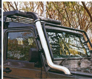
(Above) A snorkel equips the Xtreme to wade through water
