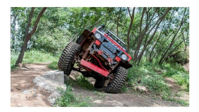
Sounds complicated? Well, I thought so too and so discovered that the best way to convey what these changes meant to the vehicle was by giving you an idea of its increased capabilities. It can now scale a gradient with a 60-degree incline as compared to the previous RFC Gurkha's 45 degrees. The approach and departure angle have increased from 50/44 to 88/58 respectively. Finally, the water wading capability has also gone up from 1000mm to 1100mm.
