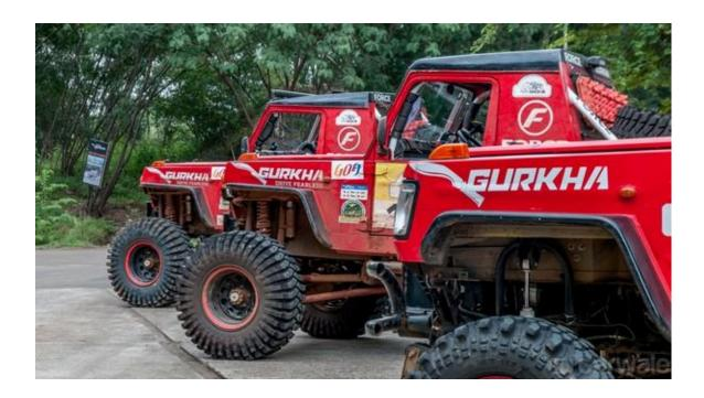
Surprisingly, the brutal diesel engine noise is produced by a stock 2.2-litre four-cylinder mill that produces 140bhp/320Nm of torque and is the same one found in the Force One SUV. The package includes a five-speed manual and locking differentials to make it a fully capable off-roading vehicle. There is a noticeable whistle when the driver gets off the accelerator and there is a snorkel intake to aid with the water wading capabilities.
